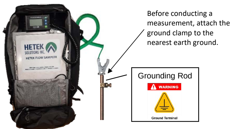
Figure 25. Hetek Flow Sampler with Grounding Clamp and Cable Assembly
